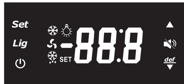
The controller has a range of 2 °C – 18 °C, with default setting of 5 °C. In order to adjust the set point please follow the below steps:
