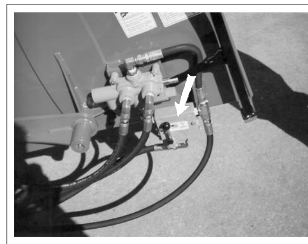
Fig. 22 FLOW CONTROL VALVE
