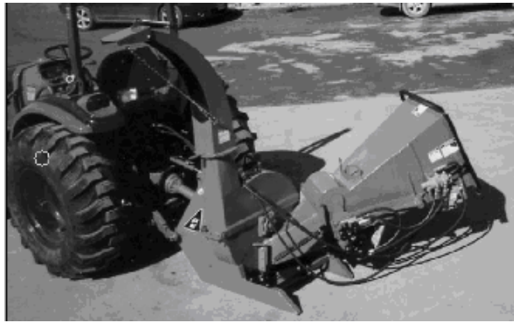
Fig. 23 FEED HOPPER/DISCHARGE HOOD
